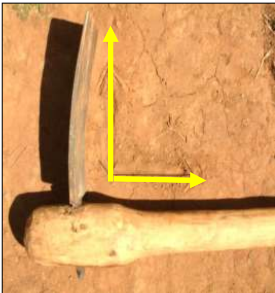
The blade must be at right angle to the shaft and fixed firmly.
