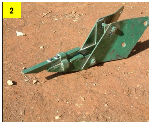
The Magoye Ripper showing reversible tine and Sub-wings
