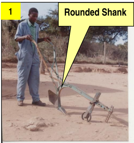
The Magoye ripper can only be fitted to plough beams with rounded shanks.
