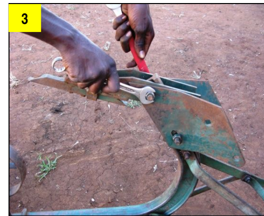
Attaching the sub-wings to the ripper tine body. Always use the correct size spanner for the job! The tine must be reversed when it gets worn.
