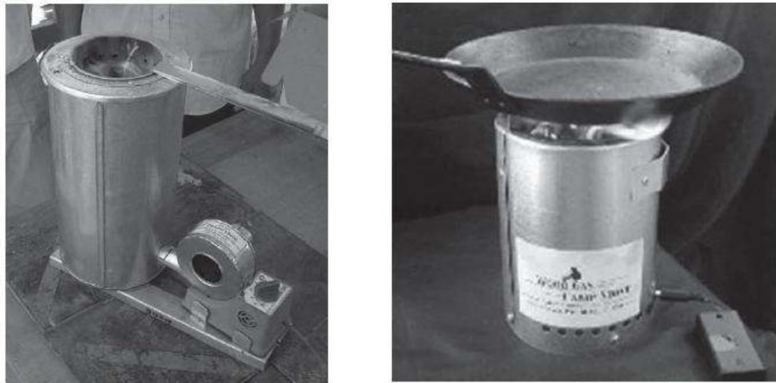
Figure 2 Reed's Woodgas Campstove (left) for sale on the Internet (US\$55) and Anderson's Juntos B+ TLUD gasifier (with removable fuel canister) hand-made in Cambodia with GERES (estimated cost under US\$20). For cooking, the pot can be placed on top of the unit or (better) be positioned on a simple pot support structure of any size so that the gasifier can be moved for refilling without disturbing the pot. (photos: Tom Reed, left, Paul Anderson, right)
