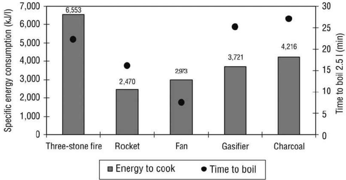
**Figure A1** Specific energy consumption (energy consumed to bring to boil 1 l water and then simmer for 30 minutes) and time to boil 2.5 l for the various stoves. Average of three tests. This chart does not include the energy to power the fan, running at 1 W for 37 minutes, or 2.25 kJ of additional energy input. Similarly, the charcoal energy consumption does not consider the energy lost while making the charcoal fuel. (MacCarty *et al.*, 2008)
