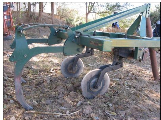
The modified 2 tine rippers in the photos above show some of the features required, but are yet to be perfected. The operating clearance of the ripper on the left is too low the coulters are set too close to the tines and the tines are too broad, whereas the ripper on the right is missing an adjustable depth wheel.
