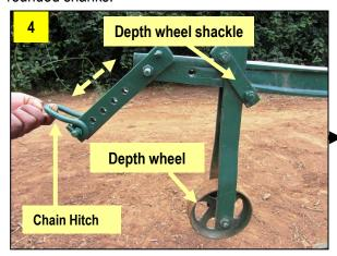
Make sure **depth wheel axle is not worn** and wheel rotates freely. Check **hitch and shackle bolts** are adjustable. Large depth wheels best.
