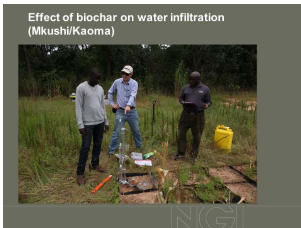
Figure 20: Measurement of water infiltration rates in Kaoma and Mkushi. The special equipment used provides an upward suction of water from the surface, lowering the pressure of the water column standing on the soil, so that the pressure of the water column is more representative of a gentle rainfall event instead of an extreme downpour (such as in the case of applying a water column without upward suction).
