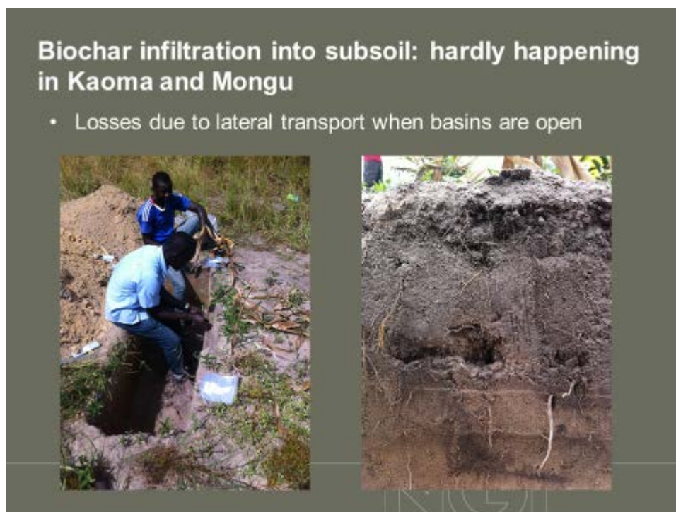
Figure 10: Soil profiles to quantify biochar leaching into the subsoil.
