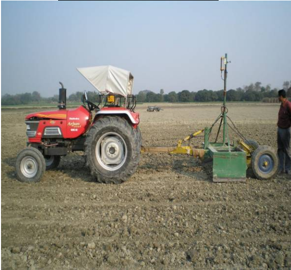
Laser-leveling in Bihar
